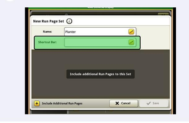
Shortcut bars can be copied and customized as desired. Ex. For a planting run page set, Operator may add planter functions like the SeedStar app and the section control master to the shortcut bar.
